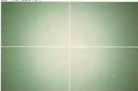
22° REFLECTOR + wide beam lens
