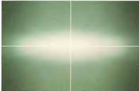
8° REFLECTOR + ellipsoidal beam lens
